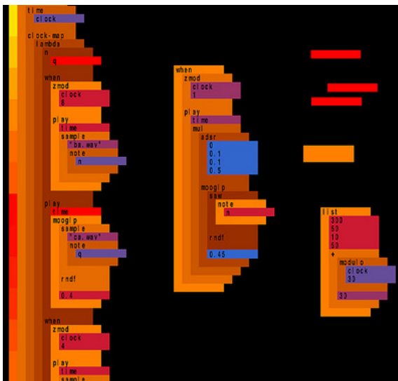
Figure 6: SchemeBricks , a lisp environment using colour instead of parenthesis, and flashes as a cue for control flow.
