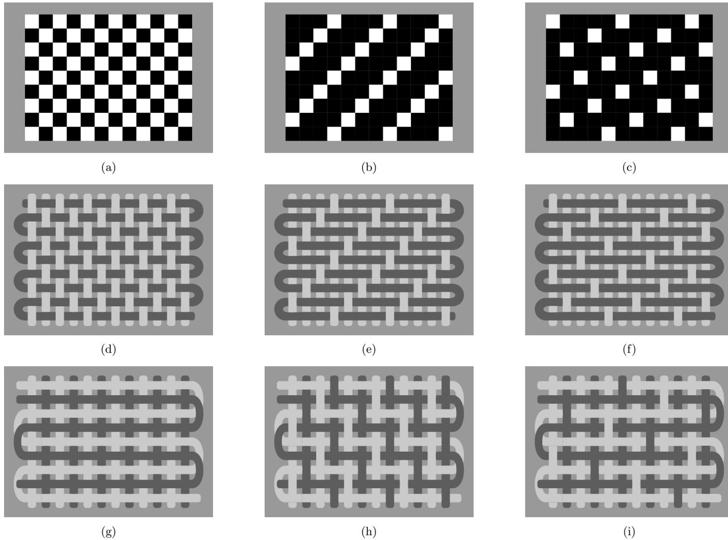
Figure 1: Fundamental weave structures, shown with binary ‘draft’ structure (top), simulated weave with light warp and dark weft (middle), and simulated weave with alternating light and dark warp and weft (bottom). These different structures lead to different physical properties and therefore uses (Emery, 2009).
