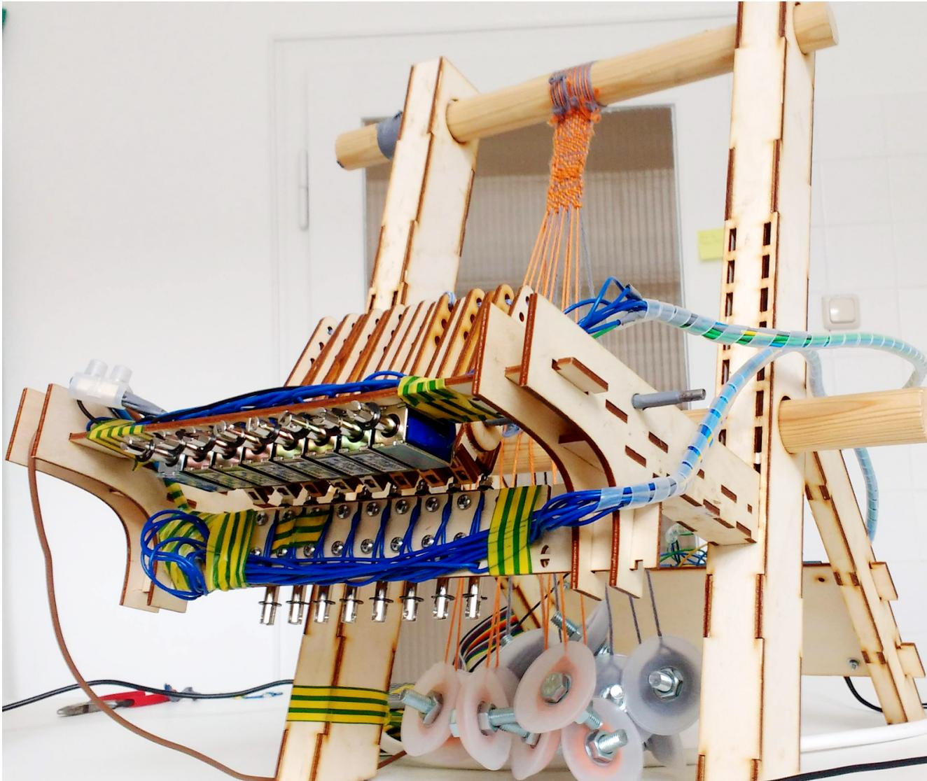
Figure 2: The Live Loom, a warp-weighted loom, with live-codeable heddles via solenoid actuators.
