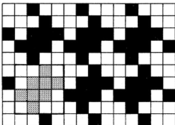
When this structure is ‘woven’ using rigid card, this does appear to be the case; half of the weave lifts off the rest, resulting in highly unstable structures:
